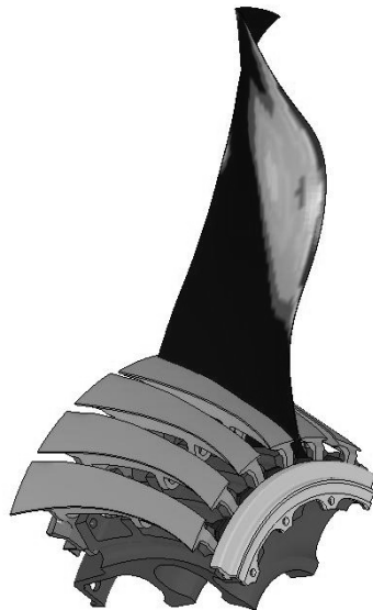
Figure 2-6: Plasticity levels on the bulge of an impacted blade.
